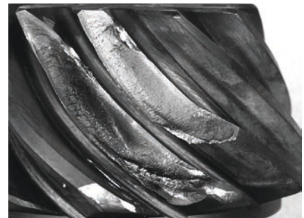
Fig. 2: Tooth fracture damage
