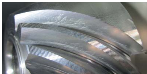
Fig. 2: Scratches on the surface during pinion cutting
